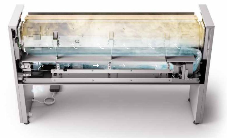
GI ironers are also equipped with a Finger-guard Cooling System (FCS), and 2 temperature sensors which, in case of overheating detected by the electronic board, intervene by switching off the heating system. A double heating activation system, with two contactors, ensures that in the event of a fault the machine is always in safety.
