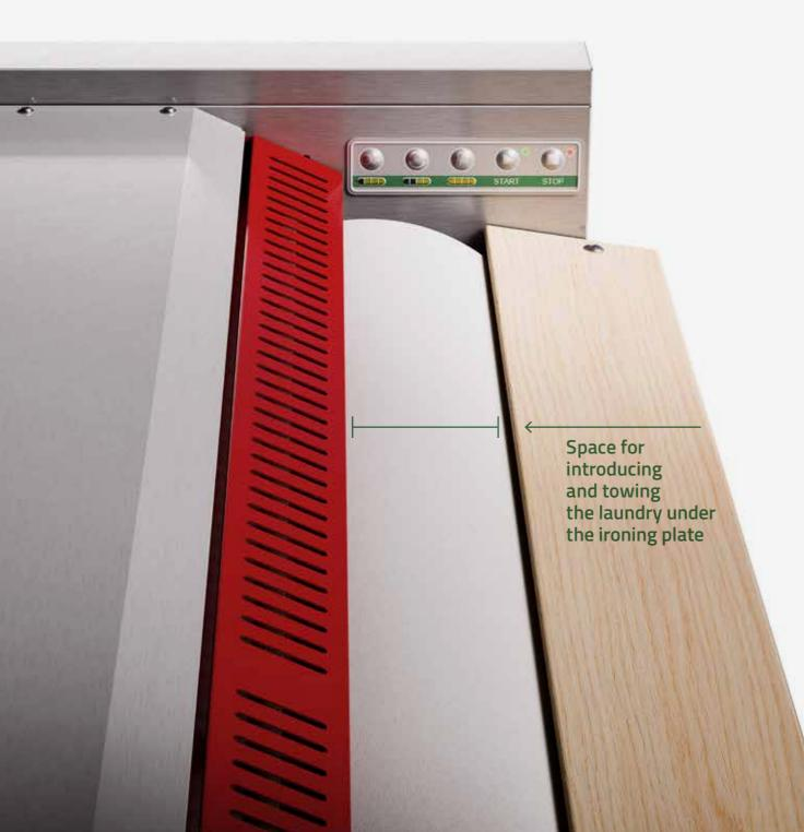
Every detail of the new **GI ironers** has been designed to provide the operator with the most comfortable working position. Such as the innovative **Adjustable Infeed Plate**: the wooden linen introduction axis, adjustable in different grades, avoids overheating and electrostatic charge.
