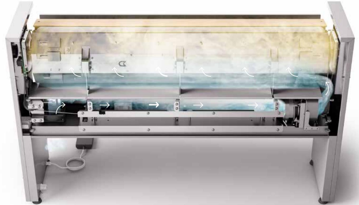
**GI ironers** are also equipped with a **Finger-guard Cooling System (FCS)**, and 2 temperature sensors which, in case of overheating detected by the electronic board, intervene by switching off the heating system. A double heating activation system, with two contactors, ensures that in the event of a fault the machine is always in safety.
